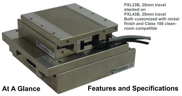
The PXL33B and PXL43B are both low profile, high precision linear motion stages. Each includes a linear motor, linear encoder and cross roller bearings with anti cage creep feature. The PXL43B can be considered the big brother to the PXL33B. The 'B' designates a different linear encoder than that used in the the PXL33A.
