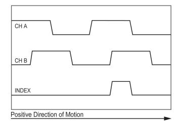
Figure 6-2: Timing diagram for the encoder signals
