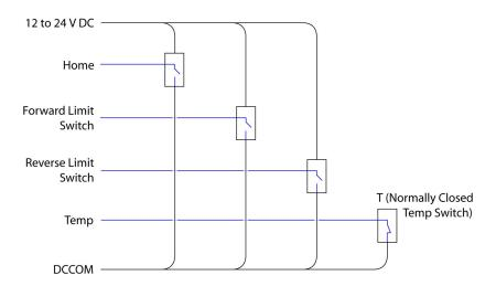
Figure 6-3: Equivalent Home, Limit and Temp Circuit Schematic
