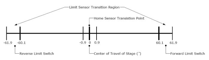
Figure 6-4: Limit and Home Sensor Transition Ranges
