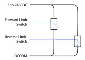
Figure 6-3: Equivalent Limit circuit schematic
