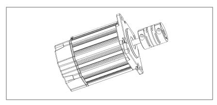
2) Slip the coupling over the ballscrew shaft and seat the motor in the motor pilot. The coupling clamp bolt should be visible. If the clamp bolt is not visible or the ballscrew shaft does not extend past the clamping bolt, repeat Step 1 and slide the coupling forward or back.
