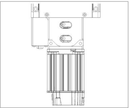
3) Mount the motor to the stage with four fasteners. Fully tighten all four fasteners.
