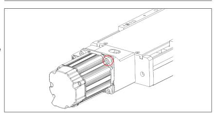
4) Make sure the coupling is not compressed axially against the shoulder on the ballscrew when the motor is seated, then fully tighten the coupling clamp screw. The coupling should be fully tightened when the coupling is in its "relaxed" state.
