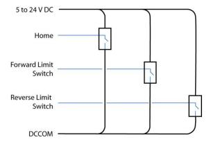
Figure 6-3: Equivalent Limit and Home circuit schematic
