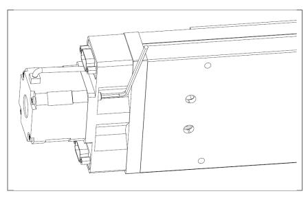
4) Fully tighten the coupling clamp screw.
