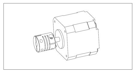
2) Slip the coupling over the ballscrew shaft and seat the motor in the motor pilot. The coupling clamp bolt should be visible. If the clamp bolt is not visible or the ballscrew shaft does not extend past the clamping bolt, repeat Step 1 and slide the coupling forward or back.
