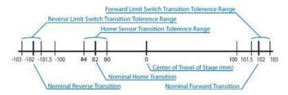
Figure 6-4: Typical Sensor Transition Regions for Default Configuration (200mm travel example)
