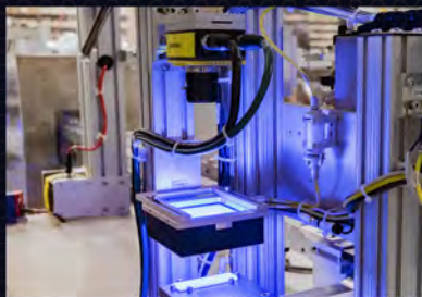
Vision inspection verifies proper strip placement
