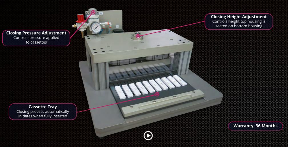
Efficient, safe and consistent closure for rapid diagnostic test strips in plastic cassettes. Closing pressure and duration is fully adjustable.
